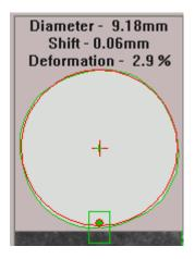
The given window displays the horizontal bullet section (green contour) obtained in the process of recording the first evolvement band, the bullet diameter value, displacement of the geometric cross-section center (green cross) relative to the rotation axis (red cross) and the bullet deformation extent (after recording the first evolvement band image), as well as the process of constructing the cross-section (by recording the first evolvement band).
