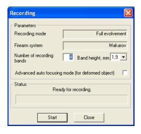
Form for the cartridge-case butt-end surfaces recording.
