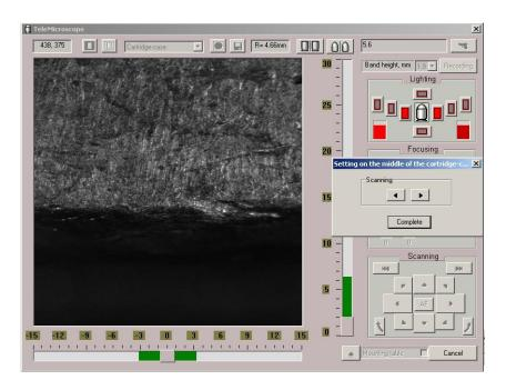
Using the navigation buttons, set the optical scanner system in a position, in which the middle of the cartridge-case edge is located over the image center, and press the **Complete** button.
