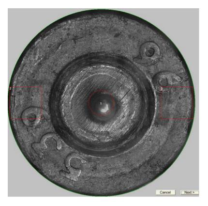
**4.** Superpose the green circumference with the cartridge-case butt-end image using the mouse. For this place the cursor inside the circumference, press the left button and move the circumference by holding down the button.
