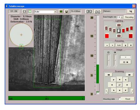
The field of image output transmitted by a CCD-camera with resolution of  $464 \times 464$  pixels onto the monitor screen corresponds to  $1.5 \times 2.0$  mm viewing field of an object.
