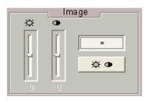
3. The "Image" tool bar contains 2 slide controls ("brightness", "contrast") and 2 double action buttons to increase the image brightness and to activate subprograms for the object images digital processing (brightness, contrast).
