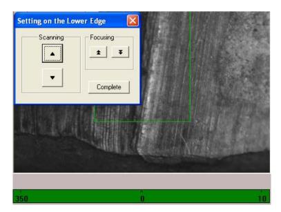
Using the navigation buttons, set the optical scanner system in a position, in which the lower edge of the object, is located in the lower part of the image window, and press the **Complete** button.
